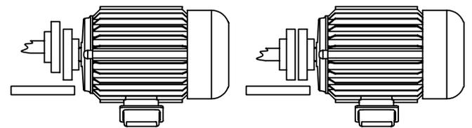
Excessive angular displacement must also be prevented. The recommended method to achieve correct angular alignment is shown below.
