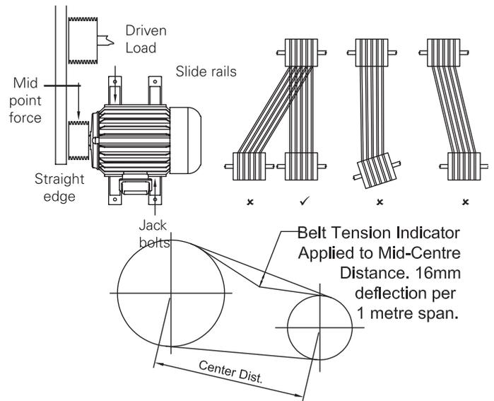
As a general rule the mid point of the applied force should be at the mid point of the shaft and it is good engineering practice to mount the motor pulley with hub and locking screw at the shaft end.
