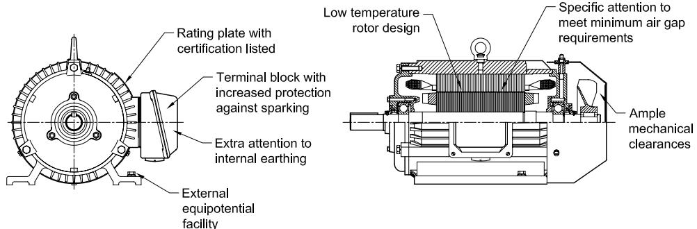
in which additional measures are applied so as to give increased security against the possibility of excessive temperatures, and of the occurrence of arcs and sparks. Ex e motors are suitable for Zone 1, Group II (A, B & C) hazardous areas, and Regal Australia provides for a temperature class of T3 (200°C) in a 50°C ambient.
