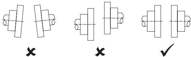
**WARNING: MISALIGNMENT OF PULLEYS WILL LEAD TO PREMATURE BEARING FAILURE**
