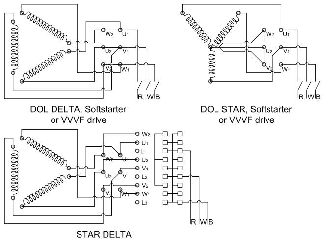
Delta with a minimum voltage of 690V.
