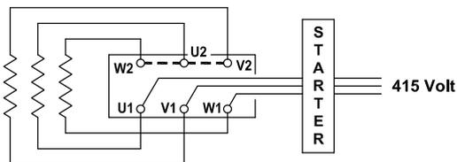
Motor connected for D.O.L. starting with bridges in place for delta connection (4.0kW and above).
