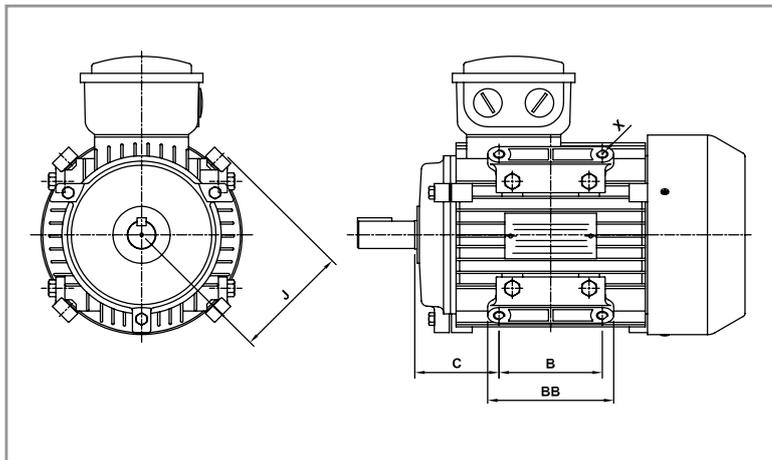
Pad mount motors are supplied by fitting 4 pads to the multi-mount motors. This option enables the mounting brackets to be fitted in a radial position relative to the motor shaft.
